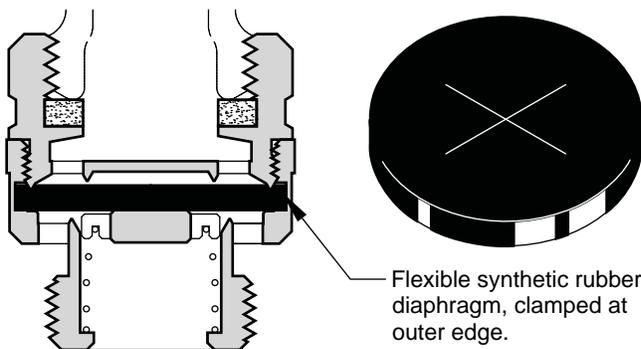
Flexible synthetic rubber diaphragm, clamped at outer edge.
